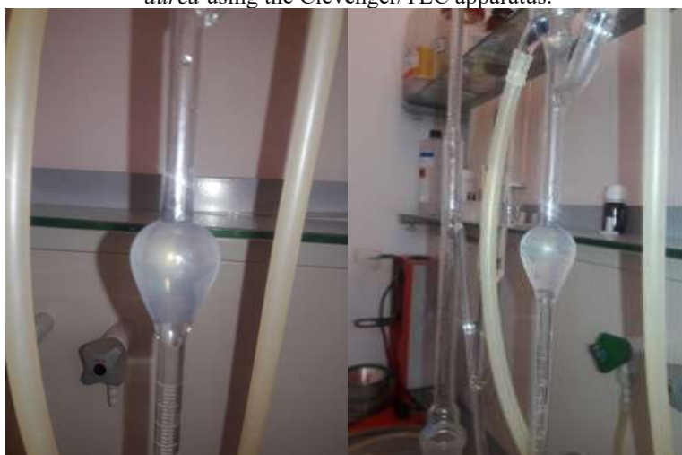
Figure 5. Magnified view of the Clevenger apparatus showing the separation and accumulation of the pale blue essential oil of Chamomilla recutita above the aqueous layer during steam distillation, confirming the formation of chamazulene.
