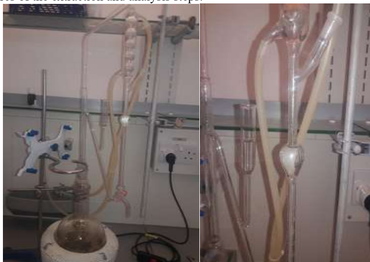
Figure 4. Photographs illustrating the steps of obtaining the pale yellow essential oil of Chamomilla aurea using the Clevenger/TLC apparatus.
