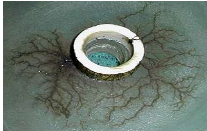
Figure 7: Treeing in underground cable insulators
