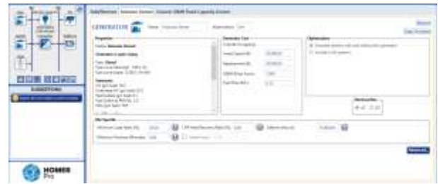
Fig. 7. Diesel-generator specification used in the source model.
