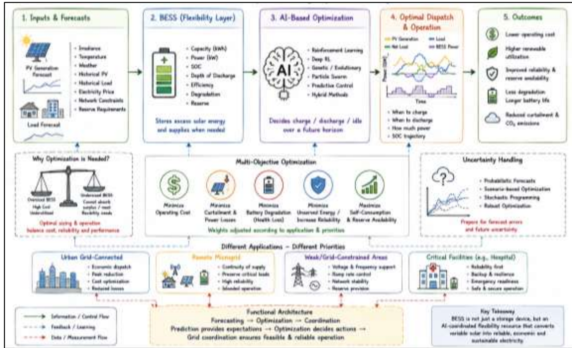
Figure 2. AI-Based BESS Optimization and Solar Energy Management From forecast to optimal storage operation and system value
